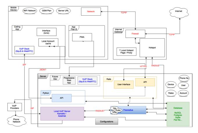
In the above diagram, the Mobile Device and Internet Gateway are separate nodes. The Server is a LibreServer base and each block is an independent application. The main Libreserver Database and Interface are placeholders that can be taken up by either the Fikelelo billing server Rails app, or the WifiCalling WebServices Server component. Work on this is ongoing, which will serve to inform a first draft standard that will be circulated for comment in a wider community.
